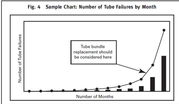
(e) Tracking of pressure loss due to tube plugging should be considered as some exchanger types cannot function properly beyond certain tube side pressure losses. Provisions for internal bypass should be considered if repair is not performed in order to prevent failure of pass partitions. Proper design of this bypass can be determined from industry references in section 7 of this Article.
