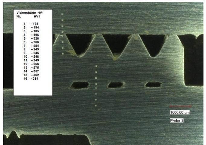
Pop-A-Plug detail of compressed internal and external sealing ring serrations.
