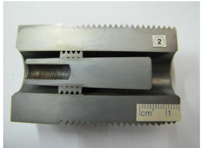
Pop-A-Plug in test coupon sectioned.
