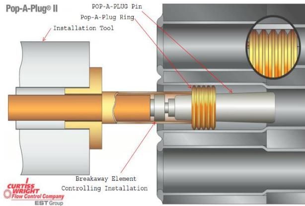
Figure 5. Pop-A-Plug® installation inside the tube inside the tube sheet
