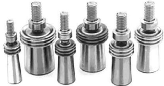
*These types of plugs have been used in services of up to 50 MPa (7,000 psi) and 595°C (1,100°F). Mechanical plugs are typically installed by a pneumatic or hydraulic system. See Fig. 3.*
