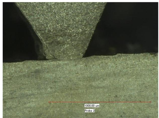
Pop-A-Plug Detail compressed tip serration.
